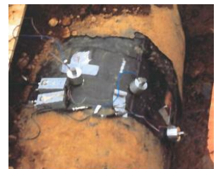
Figure 2-1. Accelerometers and Strain Gages on the 26 Inch Pipe
