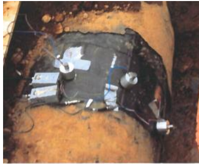
Figure 2-1. Accelerometers and Strain Gages on the 28 Inch Pipe
